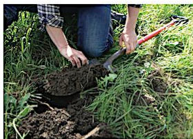
Photo 4, shaving off excess soil so that there is an even ratio of soil represented from all 6 inches of soil sampled.
