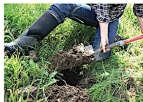
Photo 3, showing a properly retrieved soil sub-sample.
