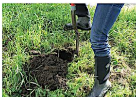
Photo 1, cutting an approximate one inch slice of soil from the side of the dug hole about 6 inches deep.
